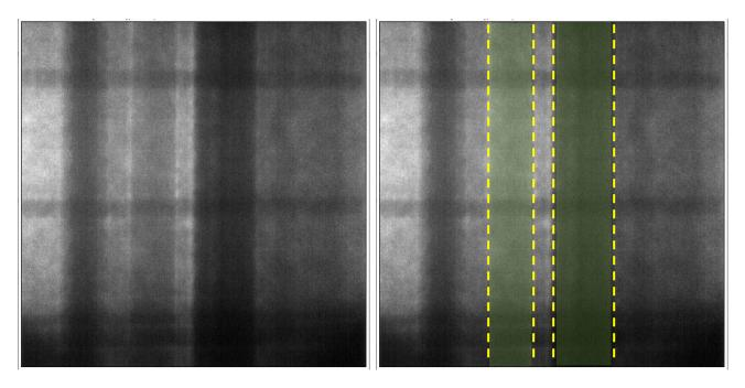
\*The areas between yellow dotted lines near the center are the PC steel bars, and the crossshaped shadows around it are the reinforcement.
